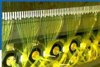
WLS optical fibers routing.
