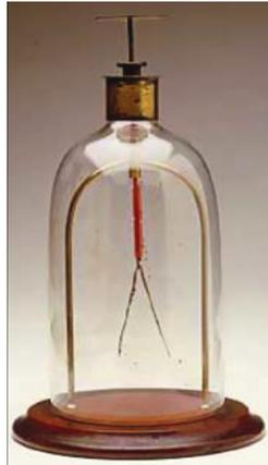
(a) A. Bennet electroscopes
