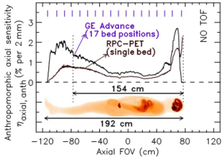
Figure 3: Anthropomorphic axial sensitivities similar to Fig. 2, but simulated with an anthropomorphic phantom adapted to Geant4.
