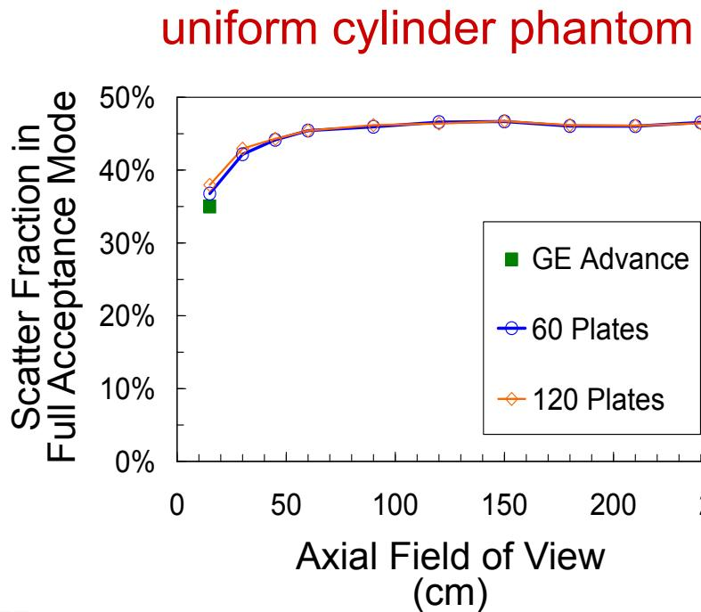
Fig. 6. Axial scatter fraction profiles obtained for the 2.4-m long RPC-PET system, and for a 17-bed scan with the GE Advance.
