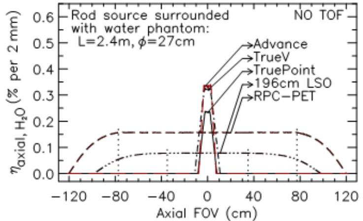
Figure 2: Axial sensitivities similar to Fig. 1, but with the line source immersed in a water cylinder with 27-cm diameter.
