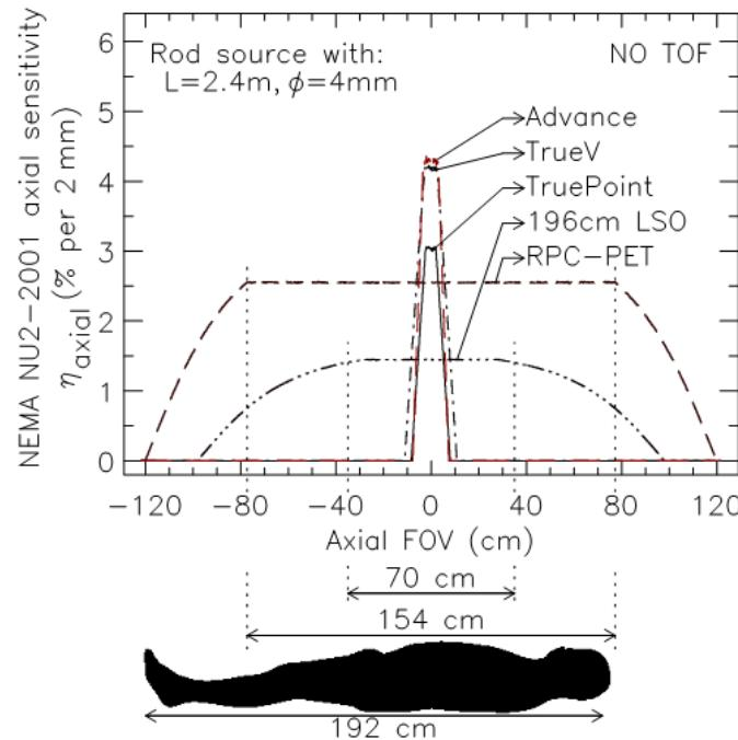
Figure 1: NEMA axial sensitivities for scanners with different AFOV. Details respecting the various PET scanners are given in Table 2. The human figure at the bottom has illustrative purposes only.
