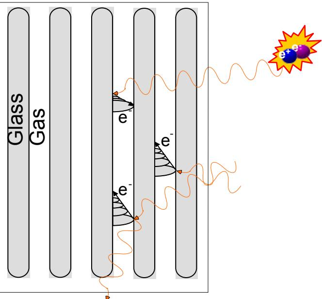
**Use the electrode plates as a  $\gamma$  converter**, taking advantage of the natural layered construction of the RPCs.
