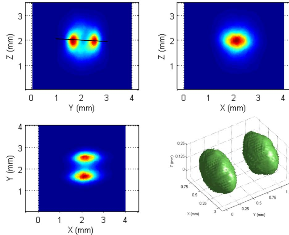
Joint reconstruction of the source in 2 positions separated by 1mm.
