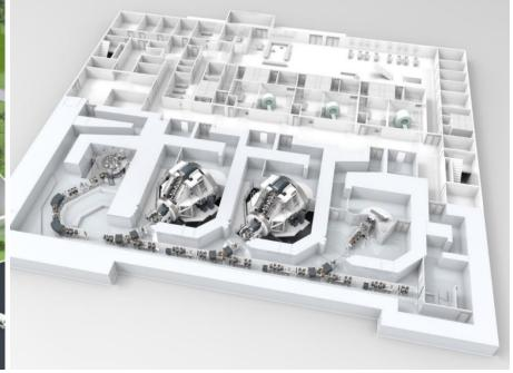
Typical multi-room configurations units for proton therapy from IBA (left) and Varian (right). These configurations can accommodate 2-3 rooms for patients and 1 room for research. Single room solutions are also available.
