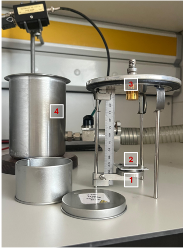
Figure 2: AEL setup. Legend: 1 – Sample holder for the source; 2 – Thin film; 3 – Silicon Surface Barrier Detector (SSBD); 4 – Vacuum chamber.
