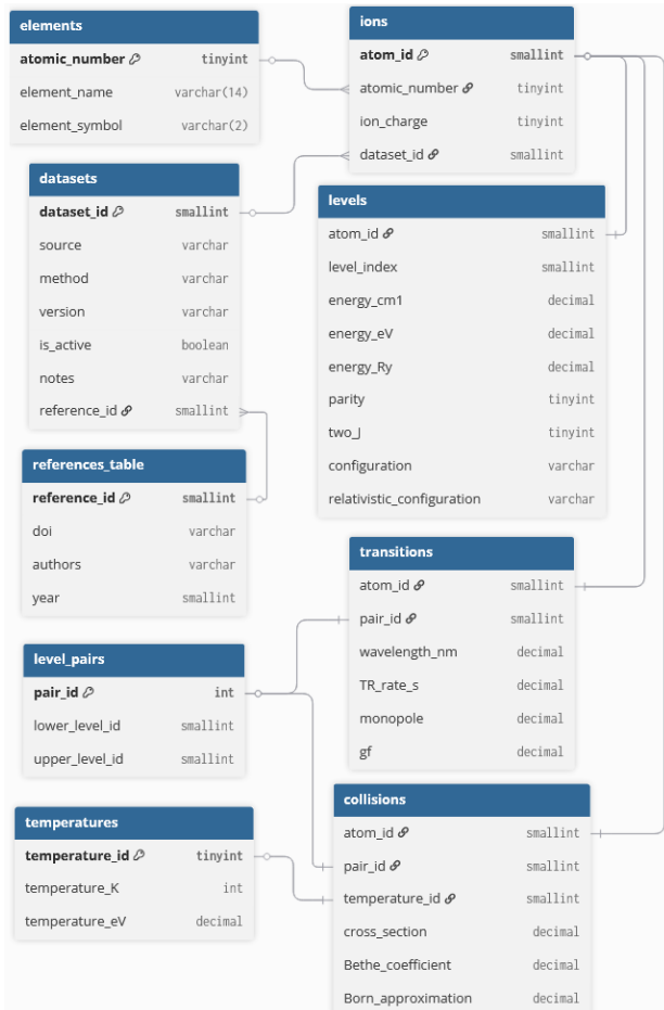
Figure 2. Schema for the DB. Schematic made with dbdiagram.io .
