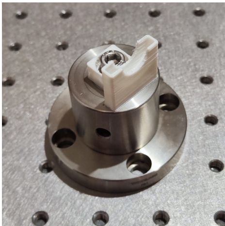
Figure 9. 3D printed adapter to the optical fiber end.
