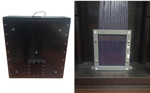
**Figure 1.** On the left, the detector as used during the laboratory essays. On the right, the scintillating plastic optical fibre array placed inside it.
