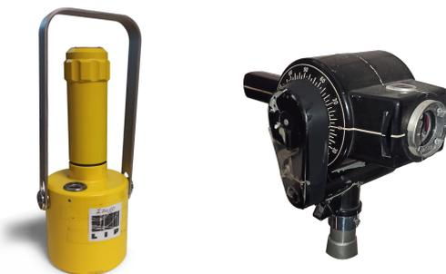
**Figure 3.** On the left, the Sr-90  $\beta^-$  radiation source. On the right, the X-Ray emitter.
