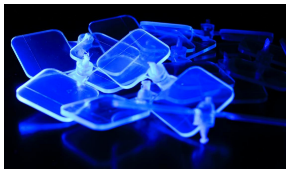
Figure 3. Scintillating PEN sample with UV light source.
