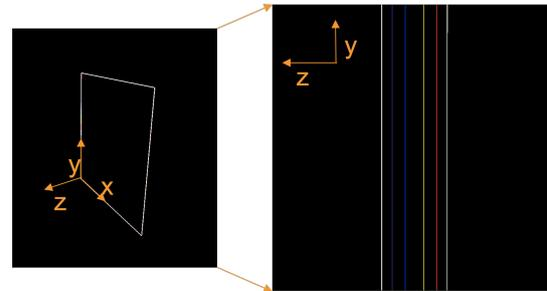
**Figure 2.** Simulation of a double nRPC detector with TOPAS. In the figure on the right, the layers from left to right are: Pickup0 (white), Glass0 (red), GasGap0 (orange), Converter0 (yellow), Cathode (green), Converter1 (lightblue), GasGap1 (blue), Glass1 (purple), Pickup1 (white). Some layers are not visible due to their width.
