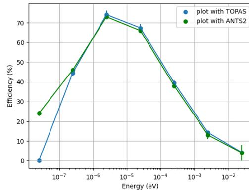
**Figure 5.** Neutron efficiency detection using the TOPAS simulation (blue) and the ANTS2 code (green).
