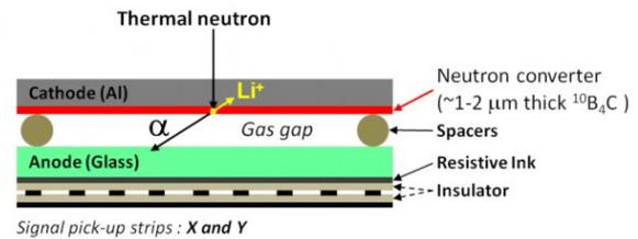
**Figure 1.** Schematic view of an nRPC detector. In addition, the process for the detection of neutrons in the converter ( $^{10}\text{B}_4\text{C}$ , red line) through the  $^{10}\text{B}(n,\alpha)^7\text{Li}$  reaction is shown.
