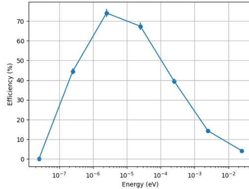
**Figure 4.** The efficiency of detection as a function of the neutron's energy. The solid line is provided to guide the eye through the points.
