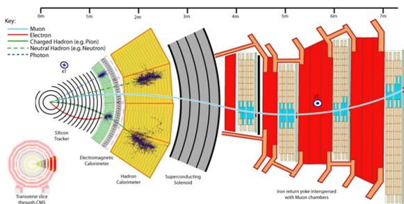
**Figure 1.** Schematic transverse view of the CMS detector
