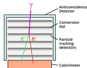
**Figure 1.** Schematic view of the LAT detector. Credits: NASA's Goddard Space Flight Center.
