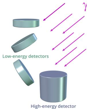
**Figure 2.** High and Low Energy detectors on the GBM face. Credits: NASA's Goddard Space Flight Center.
