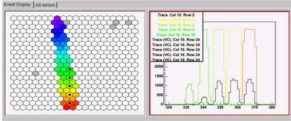
Fig. 5. Display of a simulated very high energy event: on the left the FD camera with the light track hitting the PMTs; the color scheme reflects the trigger time (blue earlier, red later). On the right the ADC traces for the 5 selected pixels. Whereas some of the normal signals are saturated the associated virtual channel keeps both amplitude and charge information.
