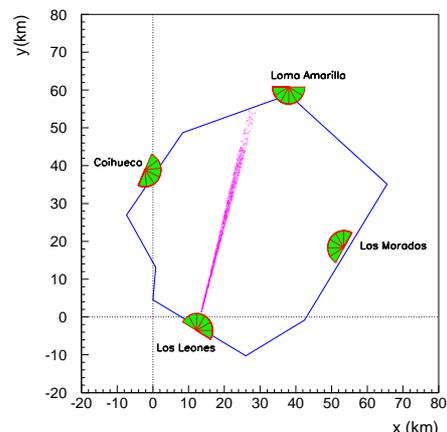
Fig. 1. A sketch of the Pierre Auger Observatory showing the core positions of the simulated showers. The showers have been generated in a slice of  $2^\circ$  in the field of view of Los Leones Eye Bay 4, with uniformly distributed core distances
