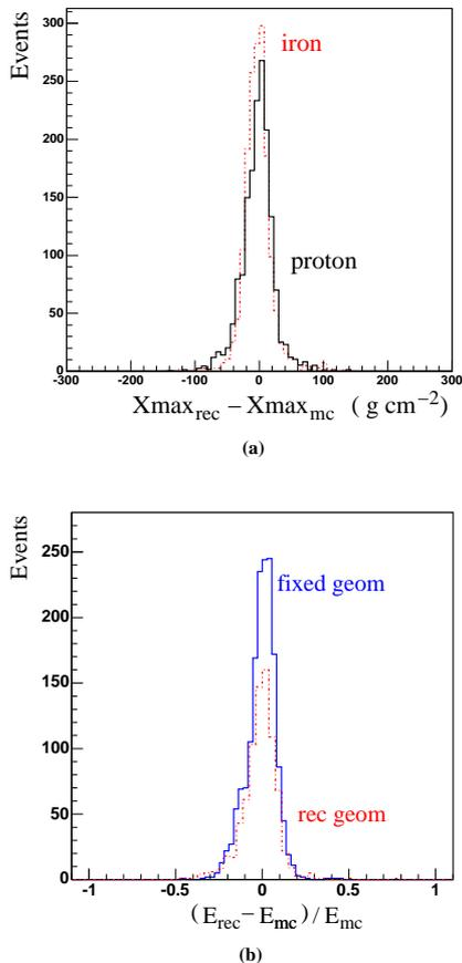
Fig. 2. (a) Residual distribution of the reconstructed depth at shower maximum (reconstructed  $X_{\max}$  - true  $X_{\max}$ ) for proton (black line, RMS=25  $\text{g/cm}^2$ ) and iron (red dot-dashed line, RMS=22  $\text{g/cm}^2$ ). (b) Energy resolution for the simulated data sample with true geometry (blue line, 1607 events, RMS=9%) and reconstructed monocular geometry (red dot-dashed line, 798 events, RMS=11%). The values are obtained averaging over the entire sample.
