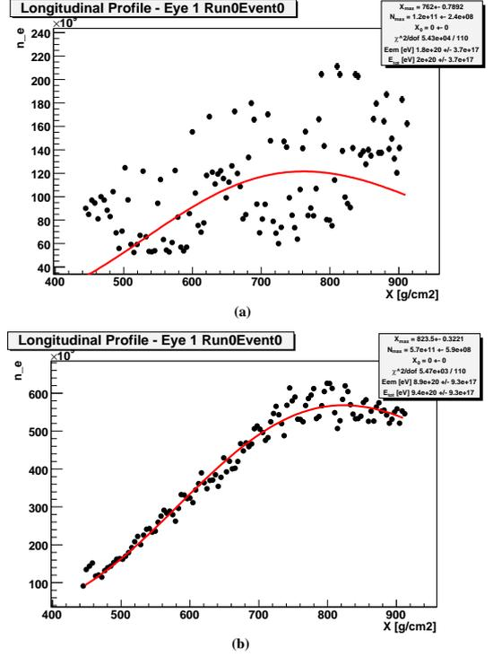
Fig. 6. Reconstructed shower longitudinal profile of an event with energy  $10^{21}$  eV and depth of shower maximum at  $825 \text{ g/cm}^2$ : top plot (a) before saturation recovery (fitted energy  $1.8 \times 10^{20}$  eV, fitted  $X_{\text{max}} 762 \text{ g/cm}^2$ ); bottom plot (b) after saturation recovery (fitted energy  $9.4 \times 10^{20}$  eV, fitted  $X_{\text{max}} 824 \text{ g/cm}^2$ ).
