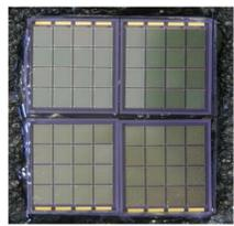
SiPM array of the camera prototype
