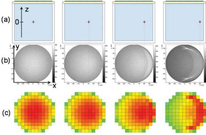
Fig. 2. (a) Scintillation position along the  $x$  axis in the middle of the crystal ( $z = 0$ ), (b) scintillation light distribution across the output window and (c) average signal detected by the elements of a SiPM array composed by 4 tiles of  $6 \times 6$  photodetectors (not fully covered at the corners).
