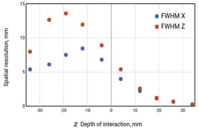
Fig. 4. Simulated spatial resolution (FWHM) along the  $x(y)$  and  $z$  directions for the events on the crystal axis.
