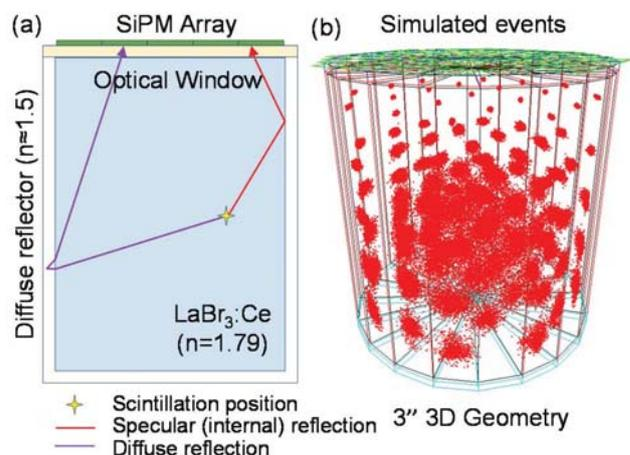
Fig. 1. (a) optical model and (b) simulation geometry of a tridimensional grid of scintillation events at 662 keV.
