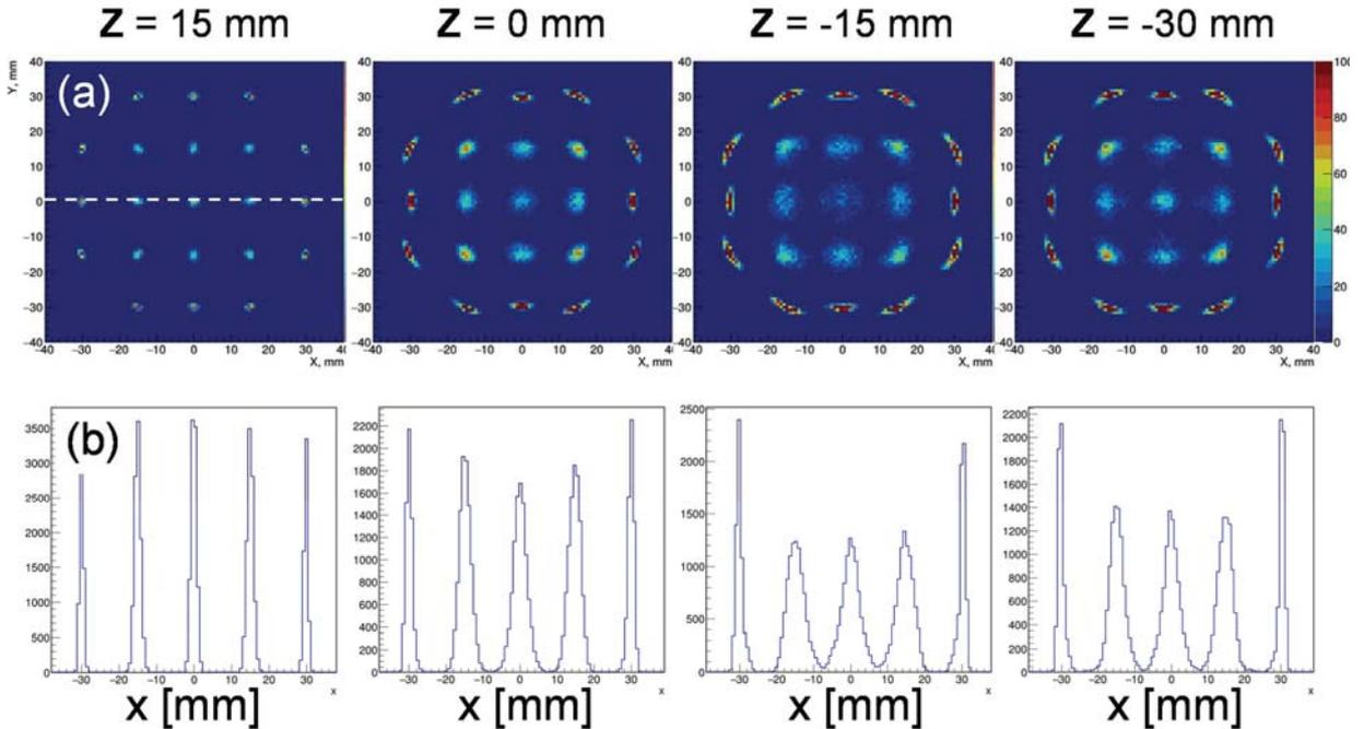
Fig. 3. (a) planar  $xy$  scatter plot of the reconstructed grid points at 4 given depths  $z$  and (b) corresponding profile along the  $x$  axis.
