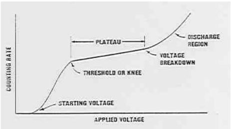
Figure 1. Typical Geiger-Mueller Characteristic Curve.
