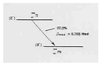
Figure 4 Beta decay scheme for <sup>204</sup>Tl.
