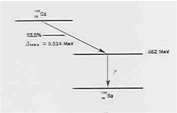
Figure 3. Decay scheme for <sup>137</sup>Cs (simplified).
