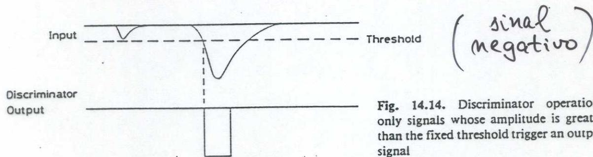
Fig. 14.14. Discriminator operation: only signals whose amplitude is greater than the fixed threshold trigger an output signal
