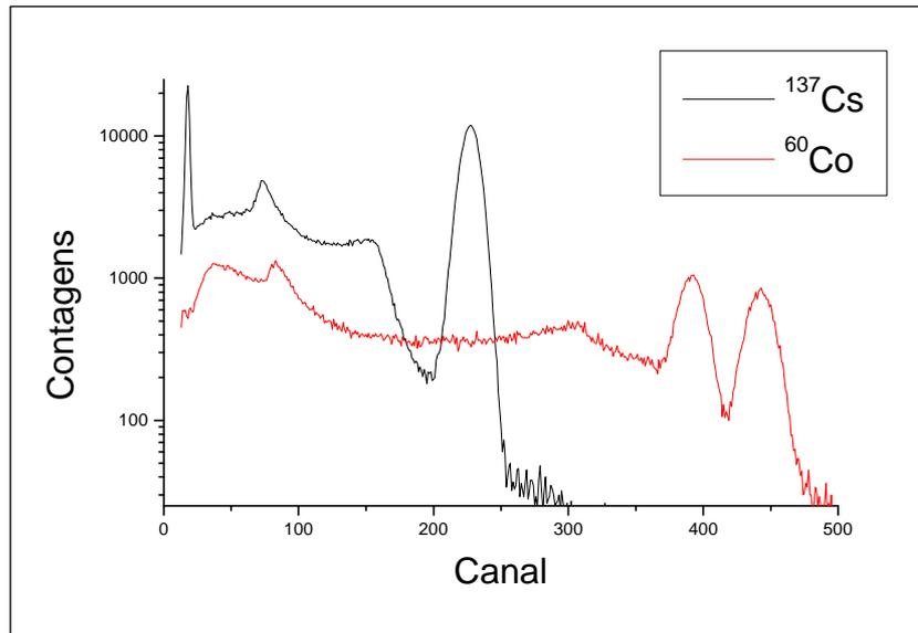
Figure 2 - Spectrum for  $^{137}\text{Cs}$  and  $^{60}\text{Co}$ .
