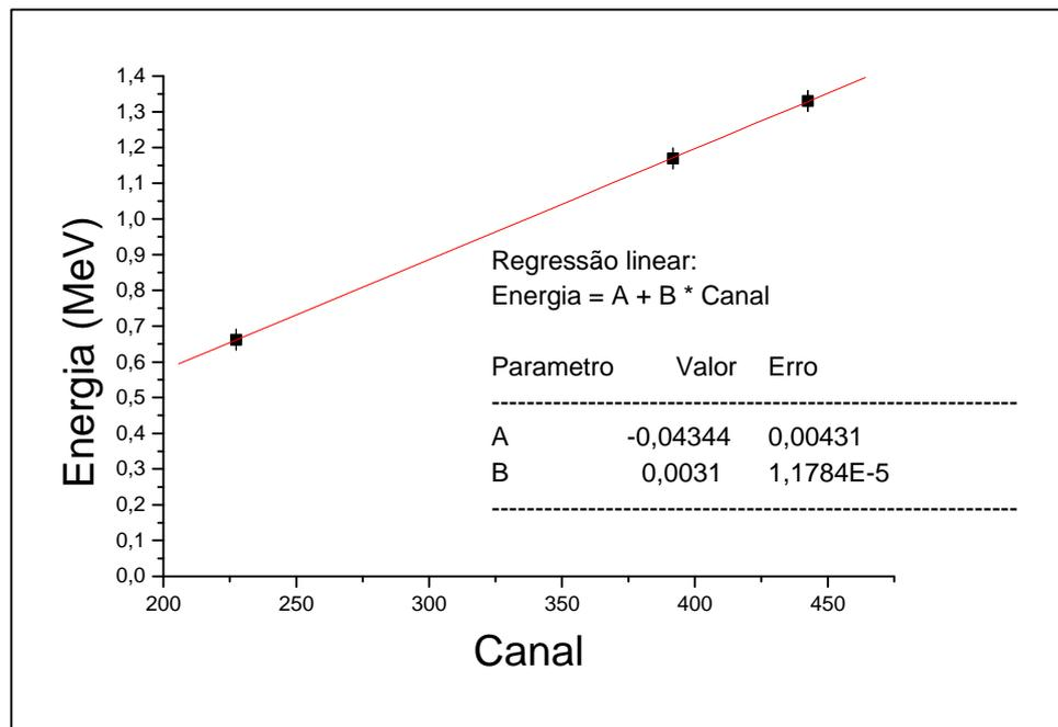
Figure 4 - Energy Calibration Curve for NaI(Tl) Detector.
