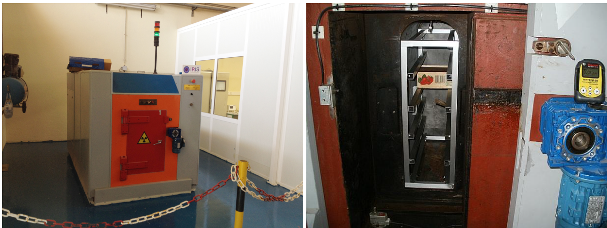
Figure 4.2: Irradiation Machine PRECISA-22, front view and inside view.
