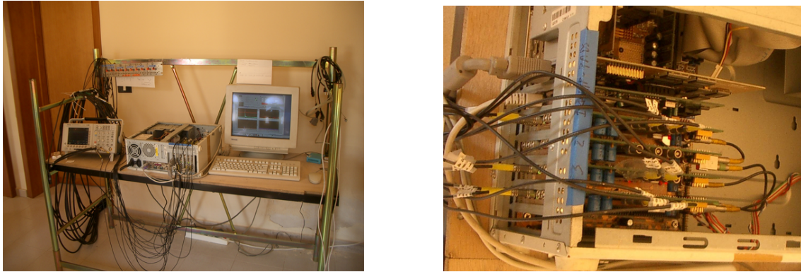
Figure 1.3: Photographs of the ULTRA DAQ at Capo Granitola. Left: Global view of the system. Signal cables arrive from the left and are connected directly to the LIP-PADS. Right: Detail of the four LIP-PADS installed in the acquisition PC.
