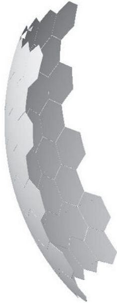
Figure 1.9: Visualisation of the Auger FD mirror as implemented in TelescopeSimulatorLX.
