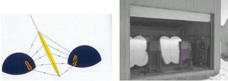
Figure 2.7: The HiRes experiment. Left: sketch of the detection in stereo mode principle. Right: photograph of one fly's eye.
