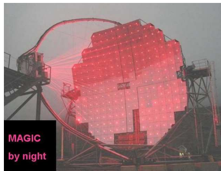
Figure 2.10: The MAGIC telescope. Here with the laser calibration system.
