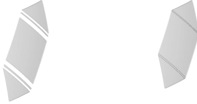
Figure 7.8: A segment of the Auger FD mirror. Left: the components of the mirror are artificially misaligned to show the internal structure. Right: the mirror segment with all segments properly aligned.
