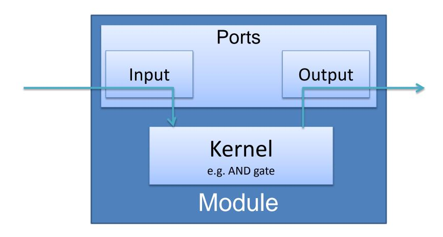
Ports in the top level module link directly to the pins
