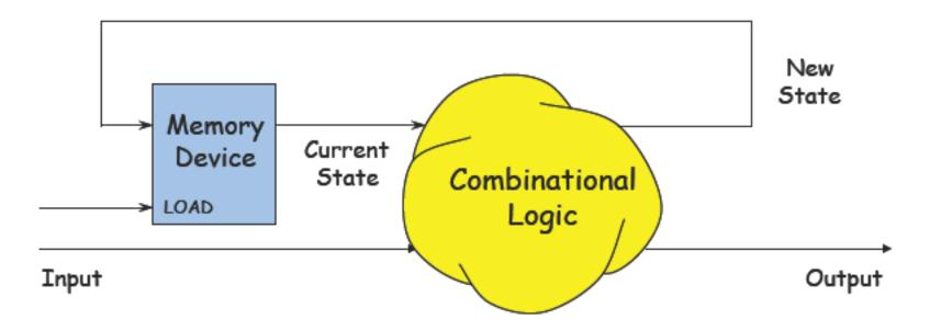
Plan: Build a Sequential Circuit with stored digital STATE -
