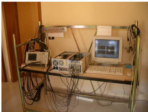
Figure 5.3: Photographs of the ULTRA DAQ at Capo Granitola. Left: Global view of the system. Signal cables arrive from the left and are connected directly to the LIP-PADs. Right: Detail of the four LIP-PADS installed in the acquisition PC.
