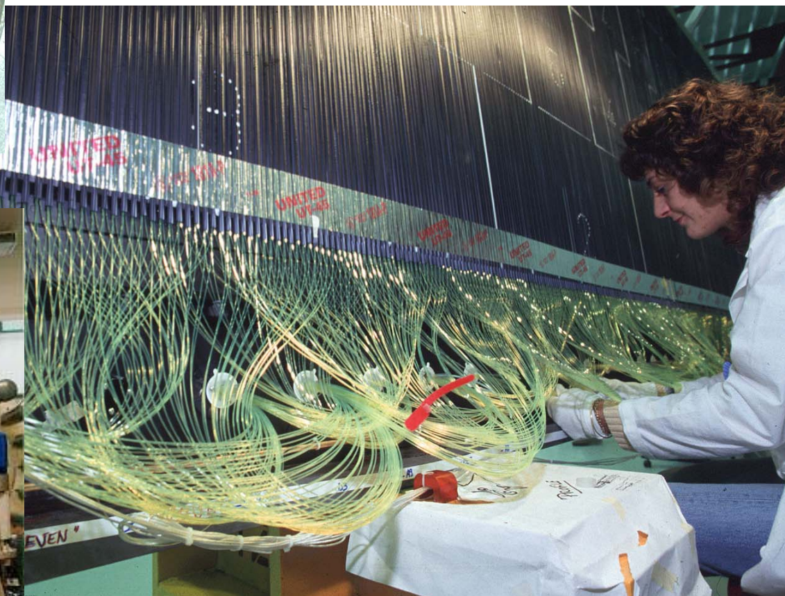
WLS fibre readout of the Tile Calorimeter
