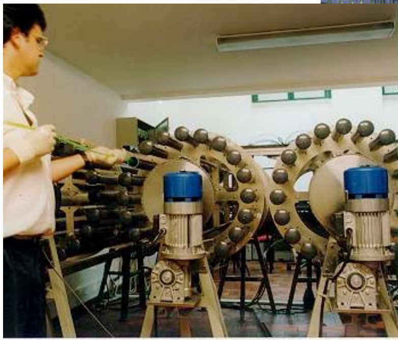
Fibres are inserted in profiles with robot
