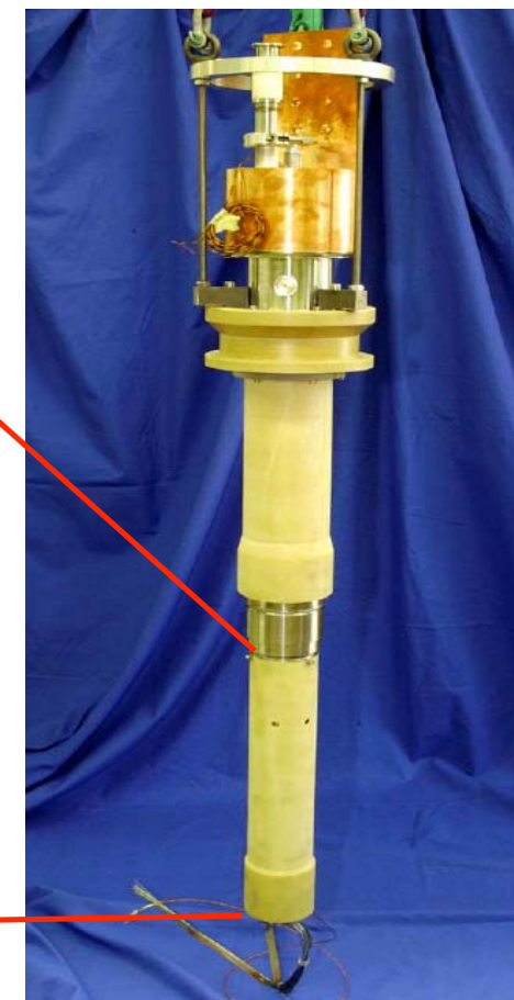
13 kA HTS current lead for LHC
