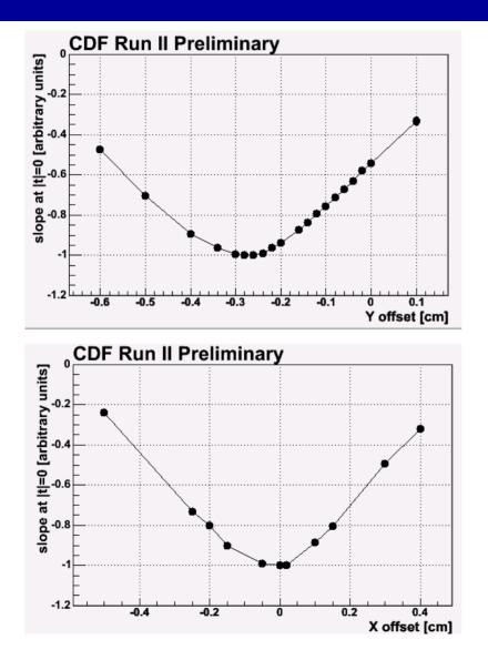
maximize the |t|-slope (normalized to max slope) ⇔determine X and Y offsets
