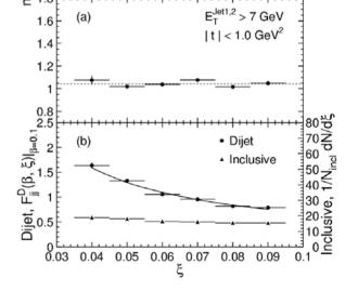
$\xi$ -dependence is IP like (m for IP is ~1.1, for IR ~0 at Tevatron)
