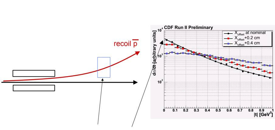
Shift detector to maximize the slope
