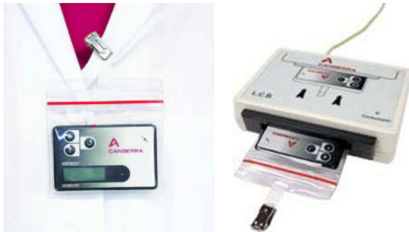
Figure 2.3: The Dosicard and the LCB badge reader. The badge has three touch buttons that allow programming and display setup on the LCD screen of the current dose, dose rate and cumulative doses per day/month/quarter/year and five years.
