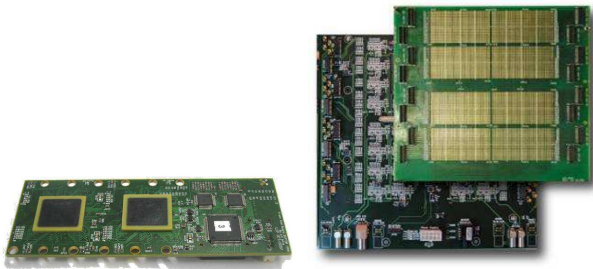
Figure 1.9: Photographs of a Front-End Board ( left ) and Service Board ( right ).
