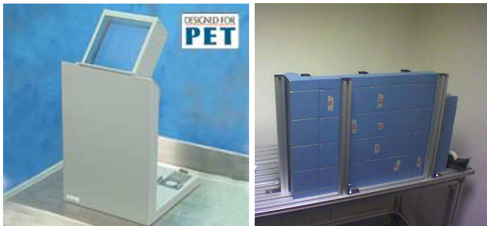
Figure 2.2: L-block table shielding for handling high-energy radionuclides( left ) and wall made of lead bricks for primary protection( right ).
