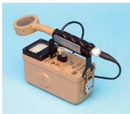
Figure 2.6: Survey Meter with Pancake GM Probe, suitable for \alpha , \beta and \gamma survey.
