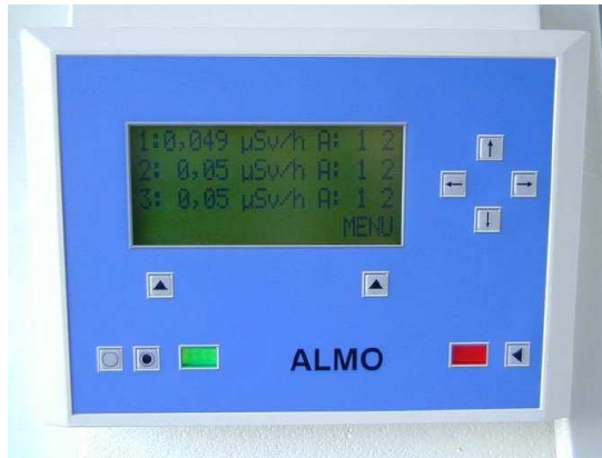
Figure 2.5: Monitor for the Almo environmental radiation control.
