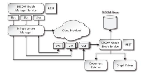
${\bf Fig.}\,{\bf 1.}$  Architecture of the graph processing framework for medical information.
