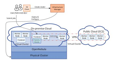
Fig. 1. Proposed cluster deployment architecture.
