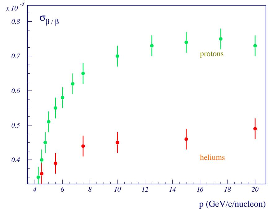
☞ the relative uncertainty on the velocity determination scales down with the number of hits
