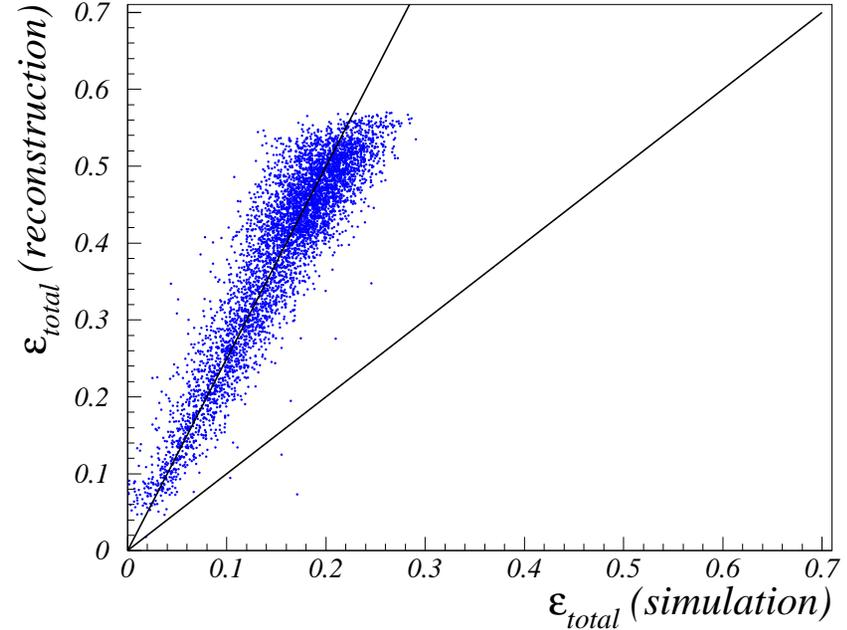
$$\epsilon_{tot} = \frac{1}{2\pi H_{rad}} \int_0^{H_{rad}} \left\{ \sum_i^{vis.paths} \rho_i \int_{\varphi_i^{min}}^{\varphi_i^{max}} e^{-\frac{d\gamma}{\Lambda_{int}}} \epsilon_{lg}\{\theta_\gamma(\theta, \varphi)\} \langle \epsilon_{pmt} \rangle d\varphi \right\} dz$$
