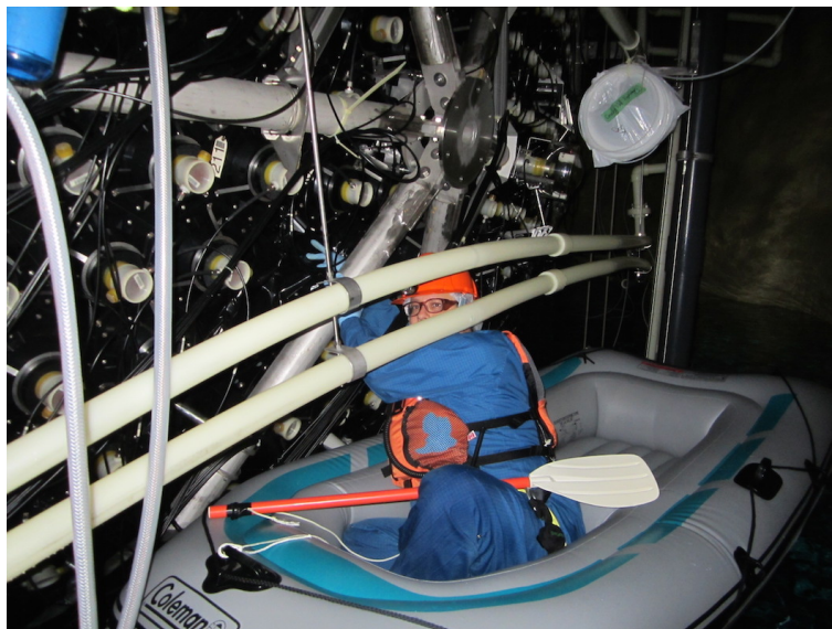
SNO+ PMT calibration system: installation of optical fibers in the detector by boat. Oct/Nov 2014.
