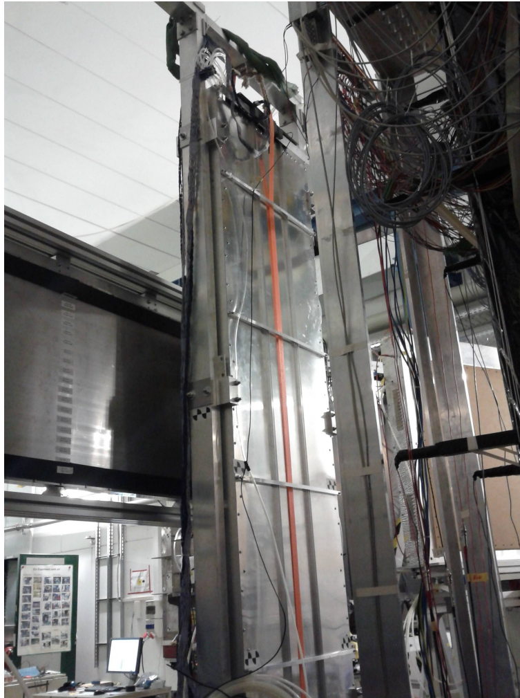
RPC prototype (vertical aluminium box) with a size of 2000 \times 500 \text{ mm}^2
