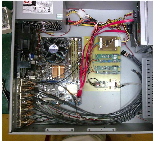
Figure 6.4: a) Front end electronics and mother boards for the RPC-PET project. b) Readout system for the monitoring of the RPC reference chambers of the RPC-TOF at the HADES experiment.
