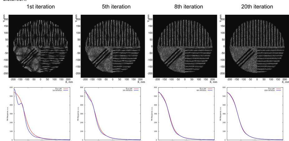
The method still works even under harsher conditions. In the example below, the photon statistics is less by a factor of two (~2000 photons per event) and the PMT gains are not equalized. Yet, after 40 iterations, the correct mask shape is recovered.
