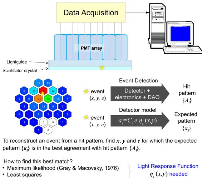
**Light Response Function (LRF)**  $\eta_i(x, y)$  characterizes response of a PMT as a function of light source position  $(x, y)$ . LRFs can be obtained from:
