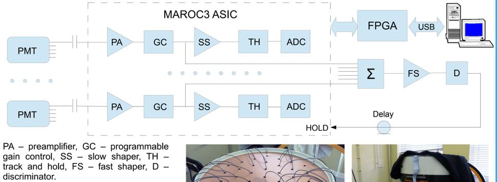
The integration time of slow shaper was set to 150 ns – maximum allowed by MAROC3 chip. Unfortunately, this resulted in sub-optimal light collection, as the decay time of NaI(Tl) scintillator is ~250ns.
