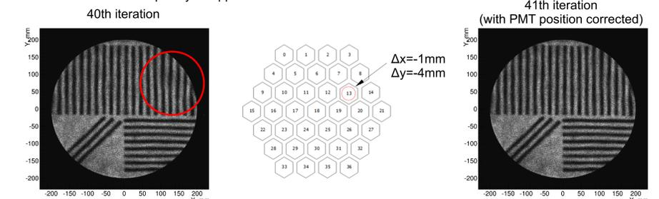
Once the LRFs are reconstructed, similar iterative technique can be used to monitor the individual PMTs for gain variations. In this case the shapes of the LRFs are fixed and only the multiplication factors are adjusted. To verify feasibility of this method the PMT gain drift was simulated by varying corresponding channel gain of the MAROC3 chip.
