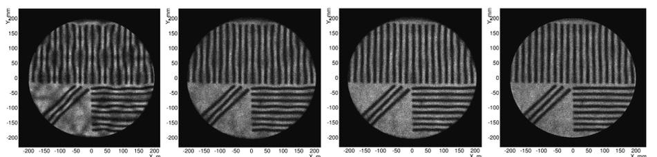
After 40 iterations almost the whole field of view becomes distortion-free except for the top-right corner. Upon individual examination of matching between reconstructed LRFs and the data, it was discovered that for one of the PMTs the axis of symmetry of the LRF does not coincide with its physical axis. After moving the axis of the LRF to the correct position the distortion almost completely disappeared.
